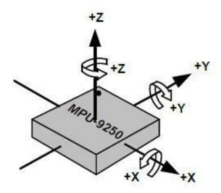
• Orientation of Axes of Sensitivity for Compass
