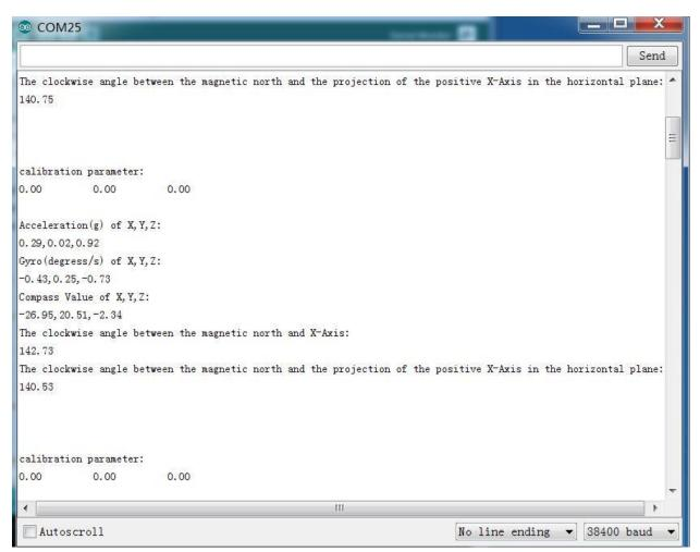
In static state, the z-Axis output value is about 0.98g, so you can refer to this to test if your sensor can work normally.
