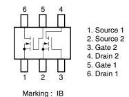
**Remark** The diode connected between the gate and source of the transistor serves as a protector against ESD. When this device actually used, an additional protection circuit is externally required if a voltage exceeding the rated voltage may be applied to this device.
