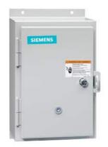
Non-reversing motor starter, Size 1 3/4, Three phase full voltage, Solid-state overload relay, OLRelay amp range 10-40a, 190 220/220 240V 50/60HZ coil, Noncombination type, Enclosure type 12, Dust/drip proof for indoors, Extra-wide enclosure
