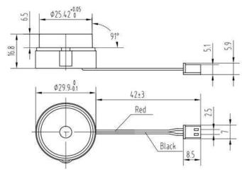
Connector Housing: A2503HOO-2P Connector crimp: A2503TOP-2
