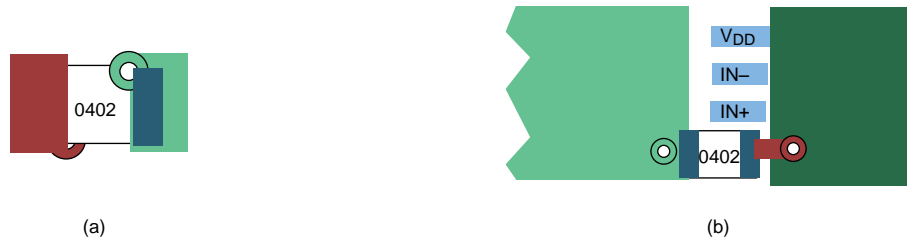
Figure 48. Typical Decoupling Capacitor Layouts
