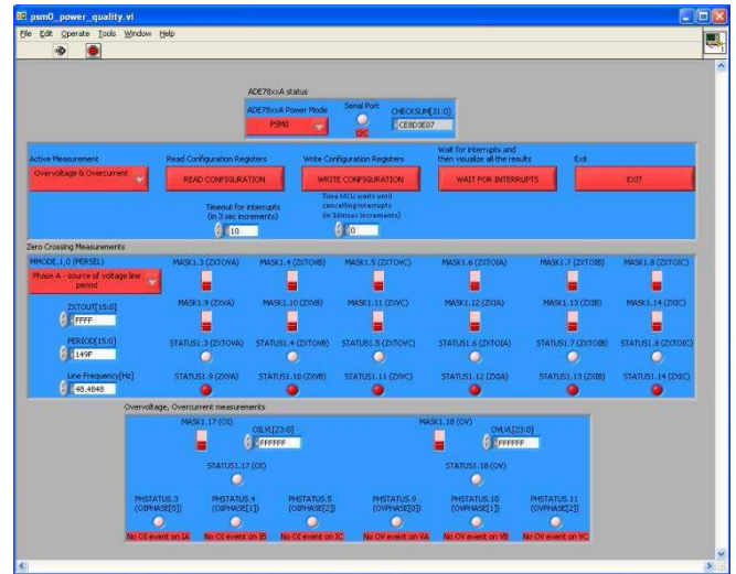
Figure 24. Overvoltage and Overcurrent Measurements Panel
