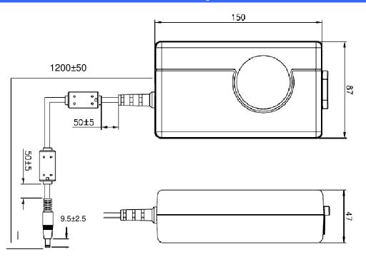
Dimensions are in mm. "#3" Connector shown.
