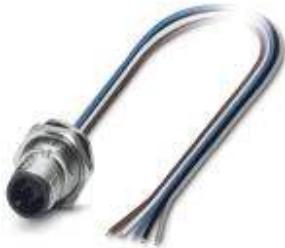
Sensor/actuator flush-type connector, 5-pos., M12 SPEEDCON, A-coded, rear/screw mounting with Pg9 thread, with 0.5 m TPE litz wire, 5 x 0.34 mm 2
