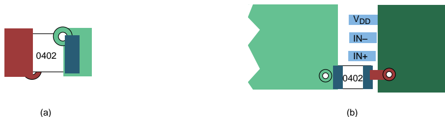
Figure 21. Typical Decoupling Capacitor Layouts
