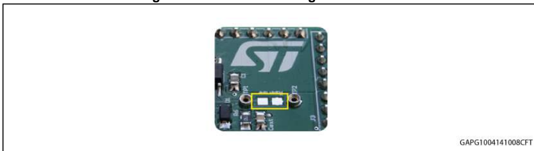
Figure 5. Pads for soldering SMD resistor
