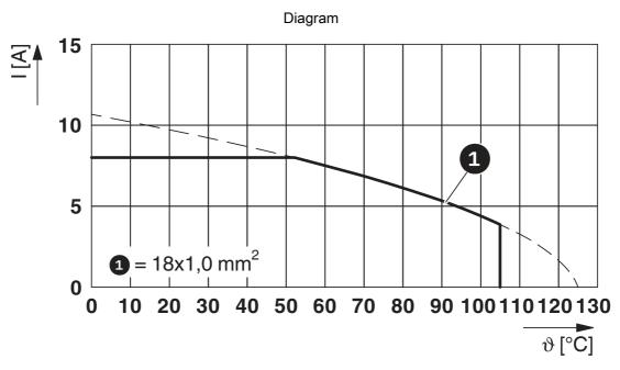
I = current strength,  $\vartheta$  = ambient temperature, 18x 8 A
