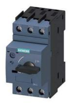
Circuit breaker size S00 for motor protection, CLASS 10 A-release 5.5...8 A N-release 104 A screw terminal Standard switching capacity Multi-unit packaging Pack = 24 units
