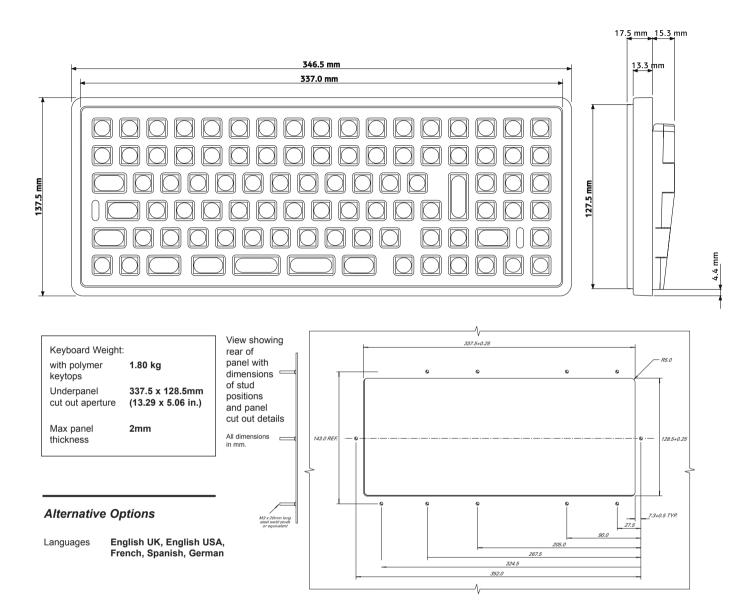
2230 Series USB 2.0 Keyboards Part Numbers White Polymer Keys, UK 2230-55201 2230-55202 White Polymer Keys, USA 2230-55203 White Polymer Keys, French White Polymer Keys, German 2230-55204 White Polymer Keys, Spanish 2230-55207
