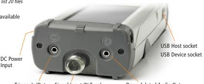
Trigger In/Out Signal Input (N Type)
