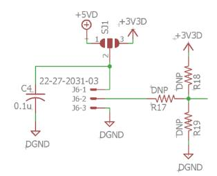
As manufactured, no I/O resistors are populated and none of the supply pins are connected. At the very least, the series resistor position will need to be populated or jumpered to gain access to the Teensy. In this example, that would be R17. These resistors and jumpers are on the bottom side of the board next to their respective connectors. Labeling is printed in the silkscreen where it could be afforded.
