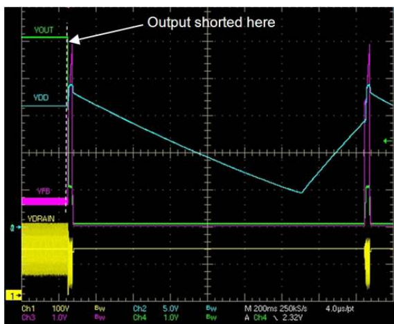
Figure 25. OLP: output short and protection tripping
