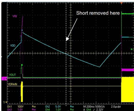
Figure 29. OLP: short removal and restart
