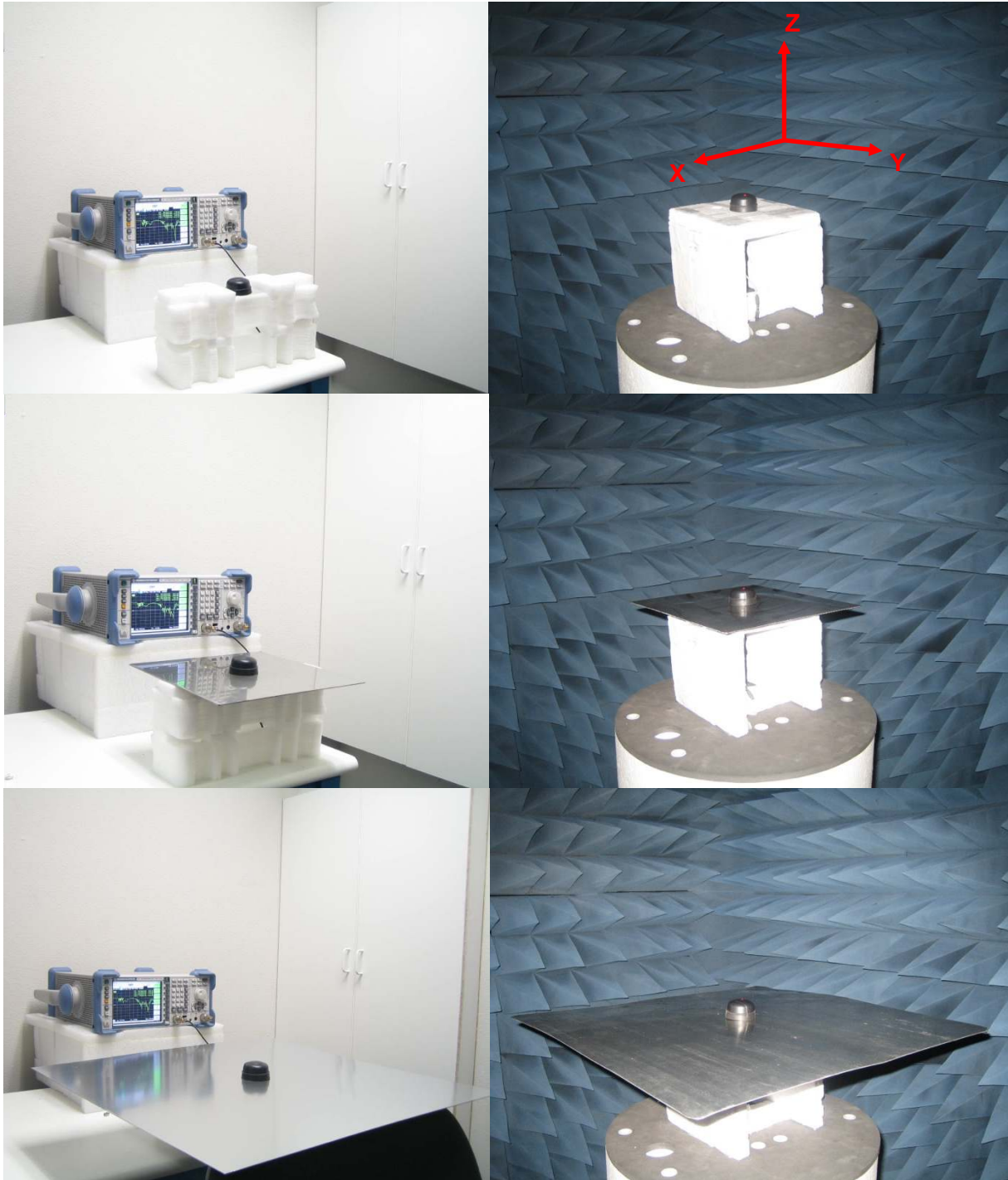
Figure 1. MA104 Antenna test set up in free space, 30x30 cm metal plate and 60x60 cm metal plate, R&SZVL6 VNA (left) and R&S4100 CTIA 3D Chamber (Right).
