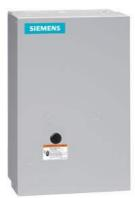
Non-reversing NEMA contactor, Size 3, Three phase full voltage, Contactor amp rating 90A, 3 wire (NO aux included), 190-220/220-240V 50/60Hz coil, Noncombination type, Enclosure NEMA type 1, Indoor general purpose use, Standard width enclosure
