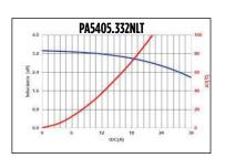
High Current Molded Power Inductor - PA5405 & PM5405 Series
