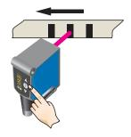
Press the Set pushbutton to end the teach-in process.
