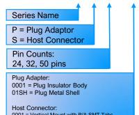
0001 = Vertical Mount with R/A SMT Tabs 0002 = R/A Mount with R/A SMT Tabs 0011 = Vertical Mount with Vertical SMT Tabs 0012 = R/A Mount with Vertical SMT Tabs
