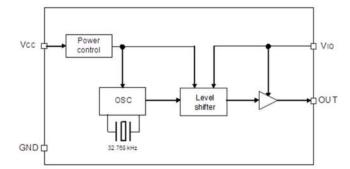
$V_{\text{IO}}$  is a power supply pin for OUT output and can also be used as an OE pin. Set  $V_{\text{IO}}$  to 0 V when setting Disable.
