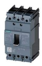
circuit breaker 3VA5 UL frame 125 breaking capacity class S 25kA @ 480 V 3-pole, line protection TM210, FTFM, In=60A overload protection Ir=60A fixed short-circuit protection Ii=10 x In nut keeper kit on both sides
