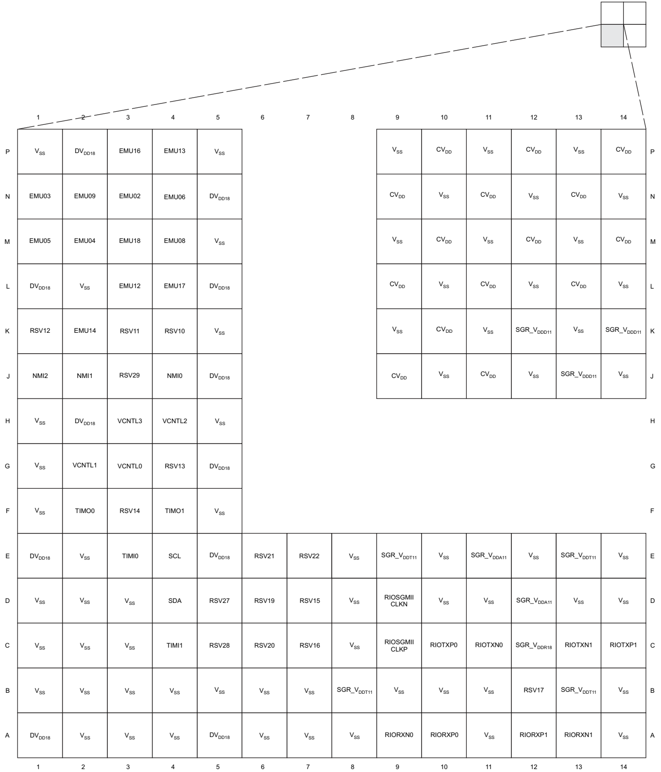
Figure 2-5. C6474 Pin Map (Bottom View) [Quadrant D]
