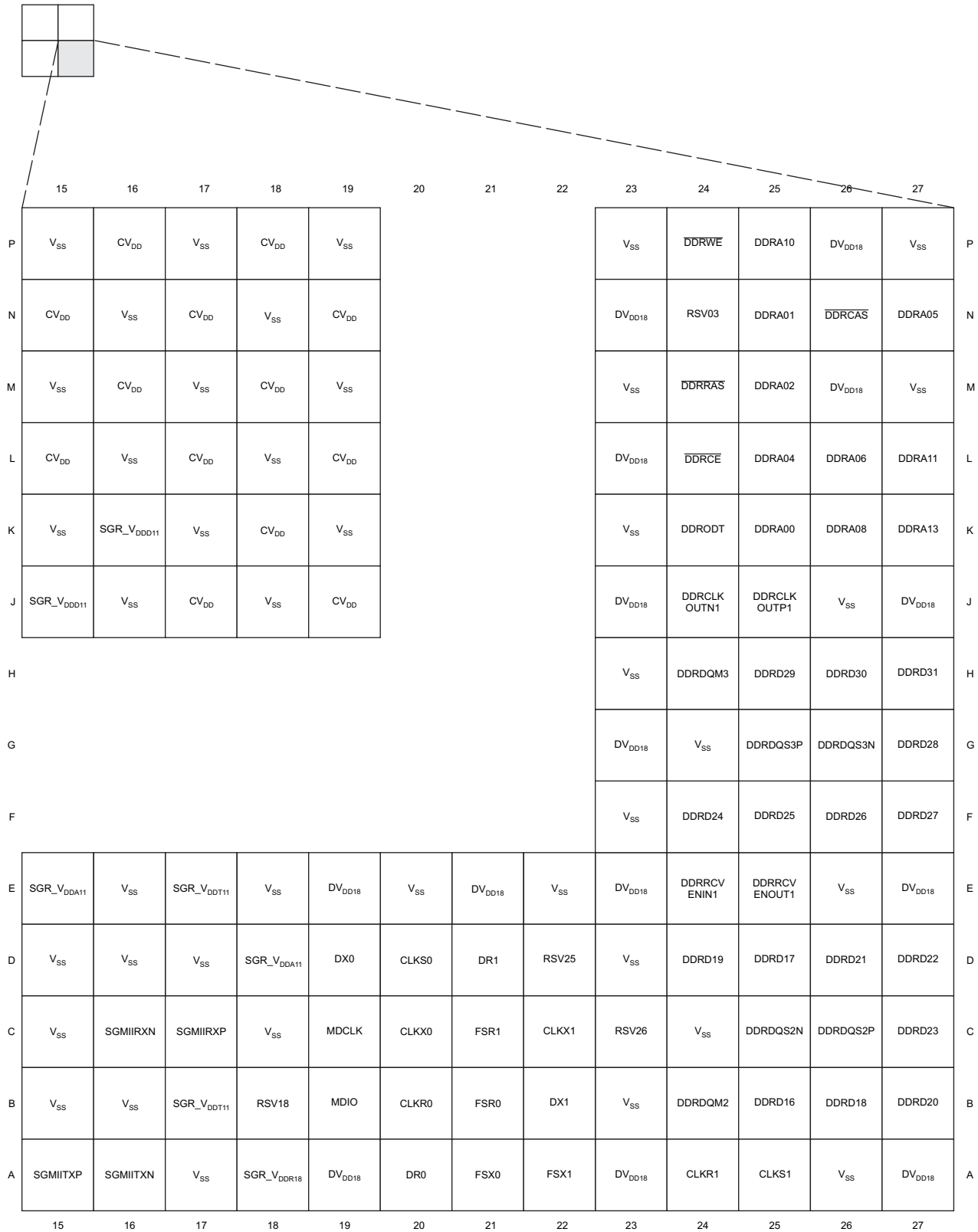
Figure 2-4. C6474 Pin Map (Bottom View) [Quadrant C]
