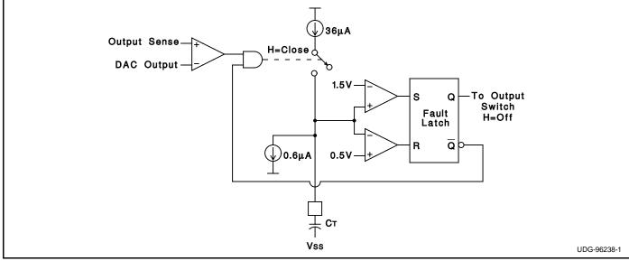
The overcurrent comparator senses both the DAC output and a representation of the output current. When the output current exceeds the programmed level the timing capacitor CT charges with  $36\mu A$  of current. If the fault occurs for the time it takes for CT to charge up to 1.5V, the fault latch is set and the output switch is opened. The output remains opened until CT dis-
