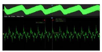
Using hardware-based Zoom technique and record length of up to 500 Mpts, users can select a slower timebase without compromising the sample rate, and then quickly zoom in to focus on the area of interest
