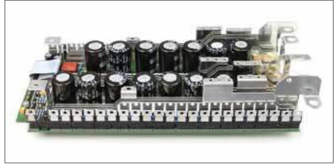
(66) Thru-hole FETs (15) High profile capacitors (9) High profile bus bars Total Weight 3.4 lbs (1543.6 g)
