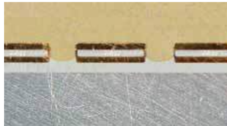
Bergquist has the ability to laminate heavy copper up to 5 oz. (175µm) on the internal layer utilizing a thicker deposit of HT dielectric.
