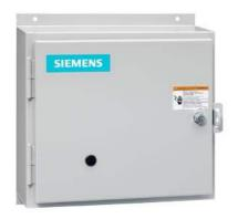
Non-reversing NEMA contactor, Size 1, Single phase full voltage, Contactor amprating 27A, 3 wire (NO aux included), 110V 50Hz / 120V 60Hz coil, Non-combination type, Enclosure NEMA type 12, Dust/drip proof for indoors, Standard width enclosure
