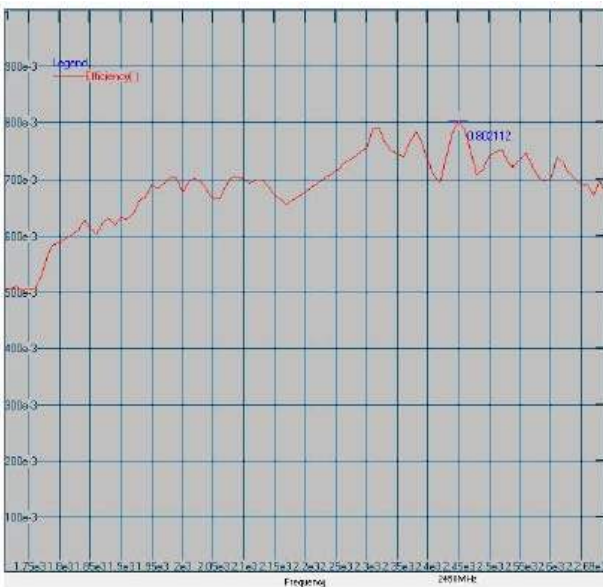
Maximum Efficiency at 2450 MHz : 80.21 %
