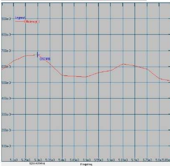
Maximum Efficiency at 5298 MHz : 67.49 %
