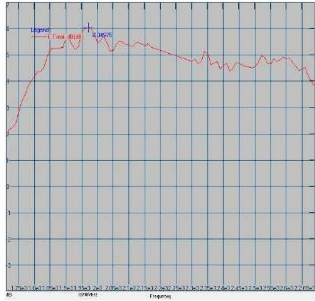
Maximum Peak Gain at 1970 MHz : 6.04dBi
