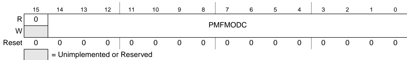
Figure 11-39. PMF Counter Modulo C Register (PMFMODC)
