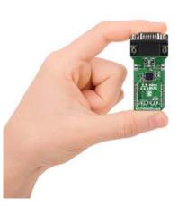
MCP25625 click is a mikroBUS<sup>™</sup> add-on board carrying a Microchip CAN controller with an integrated transceiver. It meets the automotive requirement for high speed operation (up to 1 Mb/s).
