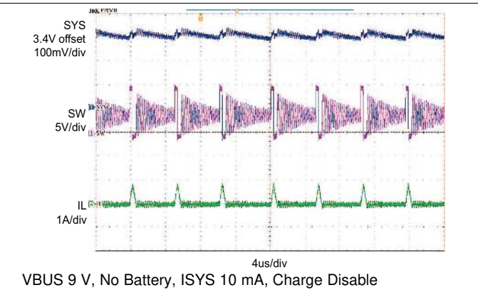
Figure 42. PFM Switching Waveform
