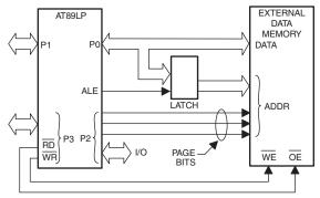
Note that prior to using the external memory interface,  $\overline{WR}$  (P3.6) and  $\overline{RD}$  (P3.7) must be configured as outputs. See Section 12.1 "Port Configuration" on page 69. P0 and P2 are configured automatically to push-pull output mode when outputting address or data and P0 is automatically tristated when inputting data regardless of the port configuration. The Port 0 configuration will determine the idle state of Port 0 when not accessing the external memory.
