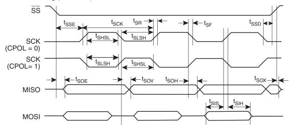
Figure 25-12. SPI Master Timing (CPHA = 1)
