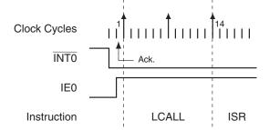
Figure 9-5. Maximum Interrupt Response Time (Compatibility Mode)
