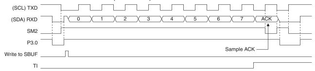
Figure 17-4. Serial Port Mode 0 (Two-Wire)
