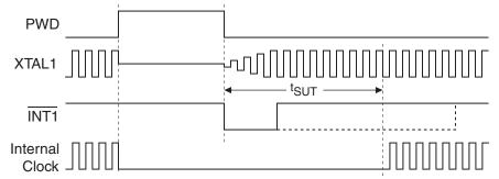
When PWDEX = "0", the wake-up period is controlled externally by the interrupt. Again, at the falling edge on the interrupt pin, power-down is exited and the oscillator is restarted. However, the internal clock will not propagate until the rising edge of the interrupt pin as shown in Figure 8-2. The interrupt pin should be held low long enough for the selected clock source to stabilize. After the rising edge on the pin the interrupt service routine will be executed.
