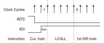
Figure 9-3. Maximum Interrupt Response Time (Fast Mode)
