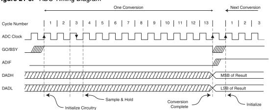
Figure 21-3. ADC Timing Diagram
