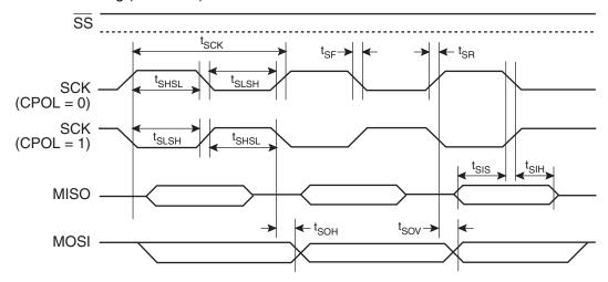
Figure 25-13. SPI Slave Timing (CPHA = 1)
