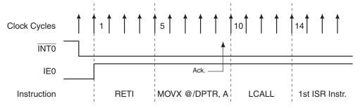
Figure 9-4. Minimum Interrupt Response Time (Compatibility Mode)
