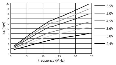
Figure 25-4. Idle Supply Current vs. Frequency
