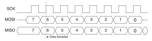
Figure 24-27. Serial Programming Interface Timing
