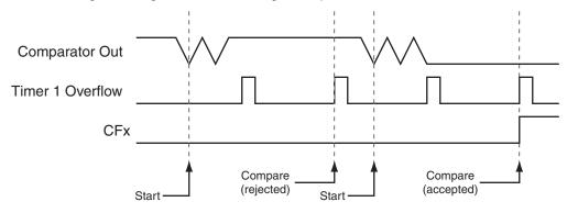
When the comparator sampling clock is configured for a timer overflow, Timer 1 still controls the debouncing. The sampling clock will determine when the edge event occurs and the interrupt will be validated two Timer 1 overflows after this event. When Timer 1 is selected for the sampling clock, this means the interrupt will occur on the second overflow after the overflow that sampled desired event.
