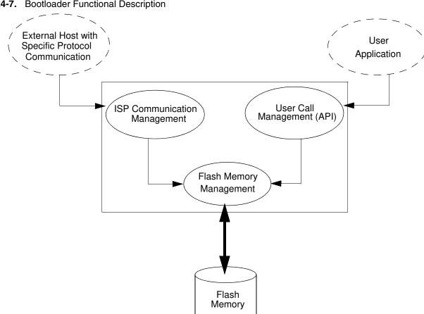
Figure 24-7. Bootloader Functional Description
