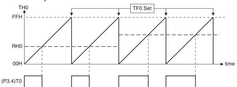
Figure 13-5. 8-bit Asymmetrical Pulse Width Modulation
