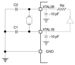
Note: 1. C1, C2 = 10–20 pF for Crystals = 10–20 pF for Ceramic Resonators
