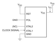
For active supply current measurements all ports are configured in quasi-bidirectional mode. Timers 0, 1 and 2 are configured to be free running in their default timer modes. The CPU executes a simple random number generator that accesses RAM, the SFR bus and exercises the ALU and hardware multiplier.
