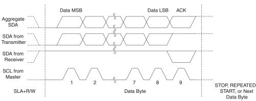
Figure 19-5. Data Packet Format
