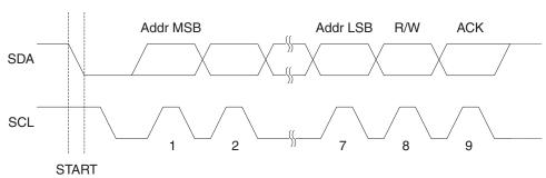
Figure 19-4. Address Packet Format
