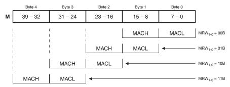
As a consequence of the MAC unit, the standard 8x8 MUL AB instruction can support signed multiplication. The SMLA and SMLB bits in DSPR control the multiplier's interpretation of the ACC and B registers, allowing any combination of signed and unsigned operand multiplication. These bits have no effect on the MAC operation which always multiplies signed-by-signed.
