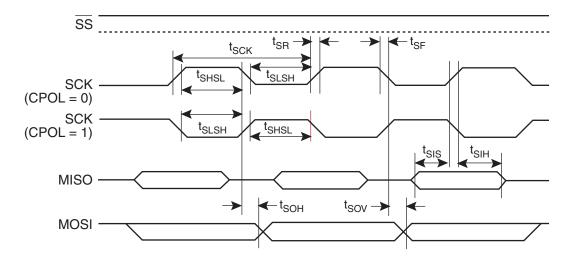
Figure 25-11. SPI Slave Timing (CPHA = 0)
