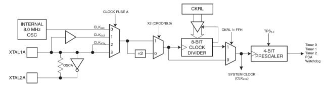
Figure 6-2. AT89LP51IC2 Clock Subsystem Diagram
