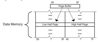
Any number of data bytes from 1 to 64 can be loaded into the temporary page buffer. This provides the capability to program the whole memory by byte, by half-page or by any number of bytes in a half-page. Note that once loaded, a buffer location cannot be reloaded with another value. The page buffer is automatically cleared after each erase/write operation.
