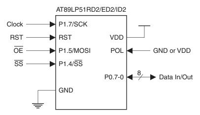
The Programming Interface is a means of externally programming the AT89LP51RB2/RC2/IC2 microcontroller. The Interface can be used to program the device both in-system and in a standalone serial programmer. The Interface does not require any clock other than SCK and is not limited by the system clock frequency. During Programming the system clock source of the target device can operate normally.
