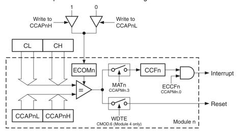
Before enabling ECOM bit, CCAPnL and CCAPnH should be set with a non zero value, otherwise an unwanted match could happen. Writing to CCAPnH will set the ECOM bit. Once ECOM is set, writing CCAPnL will clear ECOM so that an unwanted match doesn't occur while modifying the compare value. Writing to CCAPnH will set ECOM. For this reason, user software should write CCAPnL first, and then CCAPnH. Of course, the ECOM bit can still be controlled by accessing to CCAPMn register.
