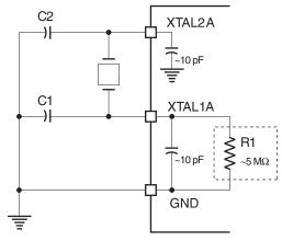
Note: 1. C1, C2 = 5–15 pF for Crystals = 5–15 pF for Ceramic Resonators
