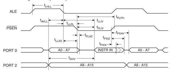
Figure 25-8. External Data Memory Read Cycle
