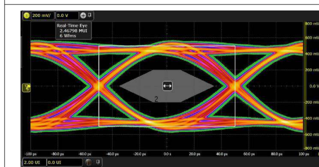
Figure 7-28. Eye at 10-Gbps Bit Rate with Increased Output Swing
