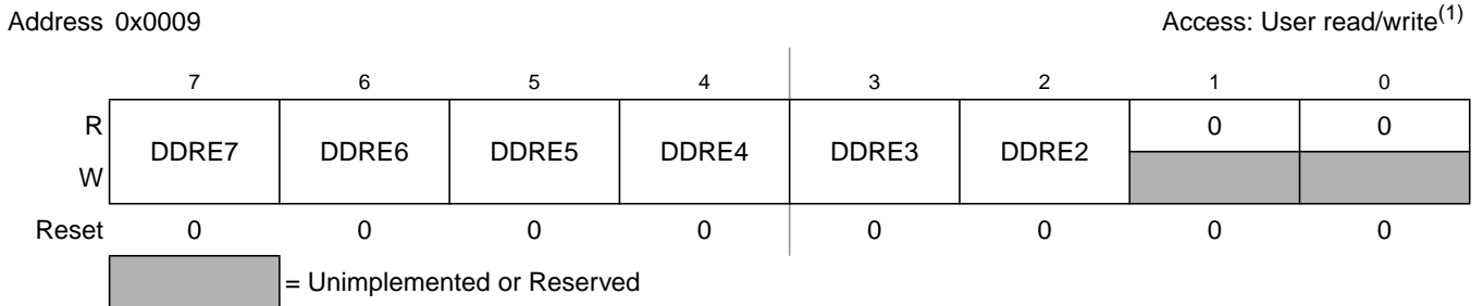
Figure 2-7. Port E Data Direction Register (DDRE)
