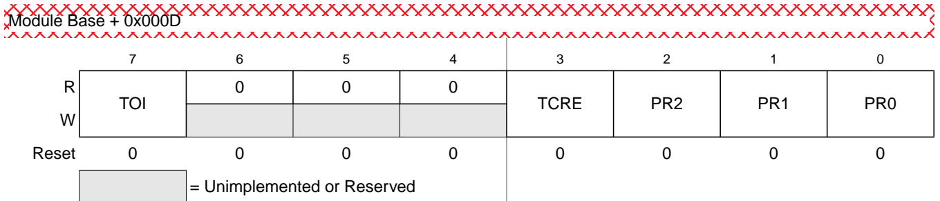
Figure 14-19. Timer System Control Register 2 (TSCR2)
