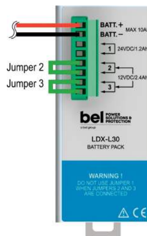
For 12 VDC / 2.4 Ah - Connect Jumper 2 and 3
