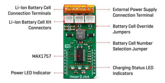
Charger 9 click requires an external power supply for its operation. To prevent an undervoltage lockout, the input voltage of the external power supply (VIN) should be at least 100mV larger than the voltage at the BT outputs (BAT pin of the MAX1757 IC). This prevents discharging of the batteries if the power source voltage drops too low. The maximum allowed voltage at the VIN terminal of the Charger 9 click is 14V, while the input current limit is set to 2A.
