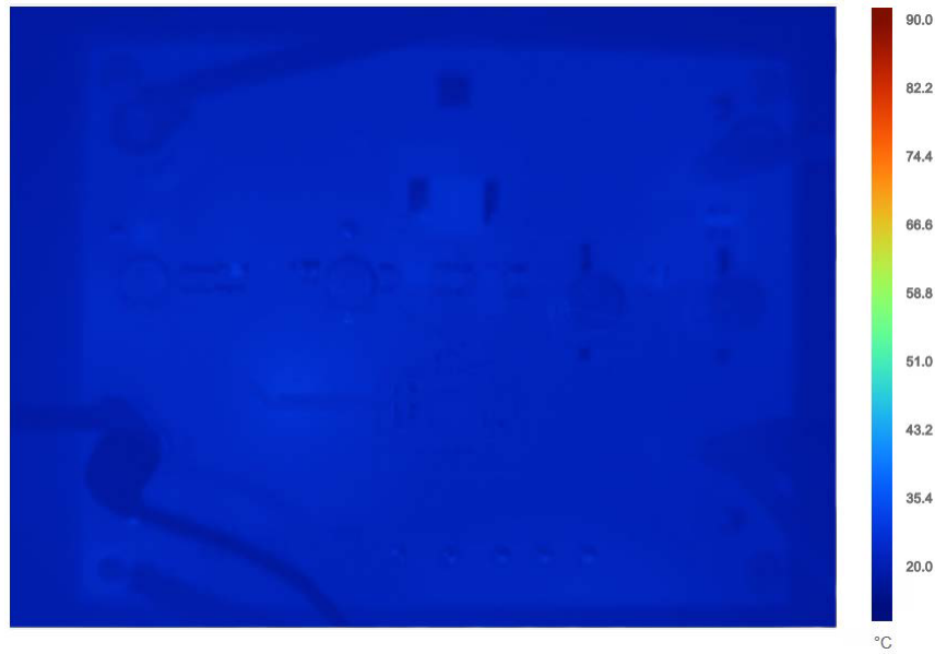
Figure 16. DC2814A-B Thermal Performance at 30V IN (Pass-Thru), 30V OUT , 2.5A Load Current
