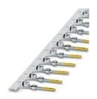
Crimp contact, Pin, rolled, Taped articles, number of pieces per reel: 10000, contact diameter: 1 mm, crimp range:  $0.22~\text{mm}^2$ ...  $0.56~\text{mm}^2$ , Item is lead-free in accordance with RoHS II without Exemption 6c (Pb <0.1%)
