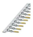
Crimp contact, Pin, rolled, Taped articles, number of pieces per reel: 10000, contact diameter: 1 mm, crimp range:  $0.08~\text{mm}^2$  ...  $0.22~\text{mm}^2$
