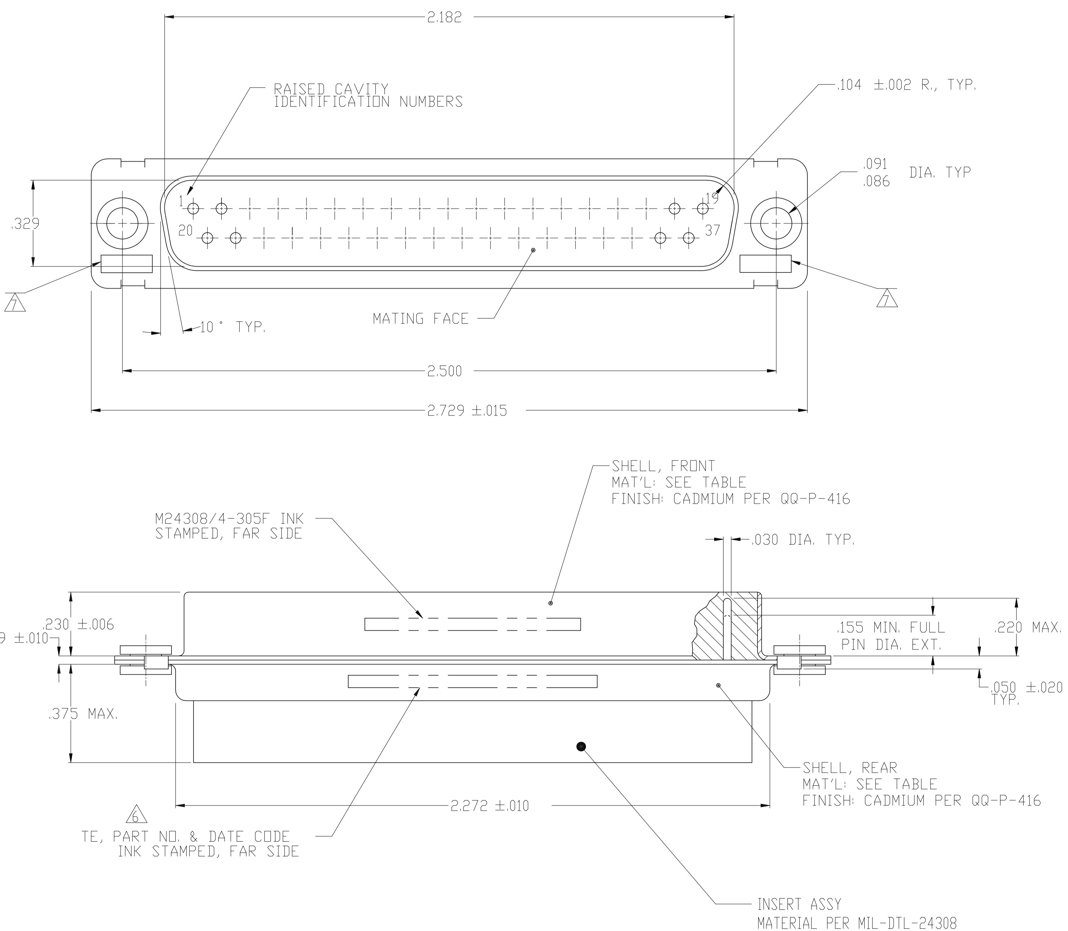
1. THIS PLUG IS DESIGNED TO CONFORM TO THE LATEST ISSUE OF MIL-C-24308
