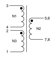
Application of the transformer allows for the leadwires between terminals 5&6 and 7&8 to solder bridge.
