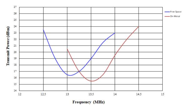
\*HF sensitivity shown in the figure is measured by Testram UD Loop Antenna 13phi. Actual sensitivity performance is subject to the environment in practice.
