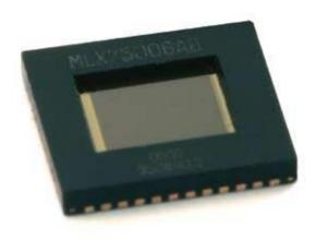
reduced costs, Melexis has developed a new signal conditioning ASIC that can be integrated with the temperature sensor in one small package. This miniature, factory calibrated temperature sensor can easily be installed by the customer on his own PCB, eliminating the need for expensive passive components and connectors. This approach allows Melexis to further standardize production and reduce cost.
