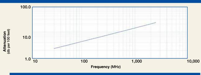
220 450 Frequency (MHz) 30 50 150 900 1500 1800 2000 5800 2500 Attenuation dB/100 ft 2.3 3.0 5.3 6.4 9.3 13.2 17.3 19.0 20.1 22.6 35.6 Attenuation dB/100 m 7.7 9.9 17.3 21.1 30.4 43.4 56.77 62.4 65.9 74.2 116.7 Avg. Power kW 0.78 0.61 0.35 0.28 0.20 0.14 0.10 0.09 0.09 0.08 0.05
