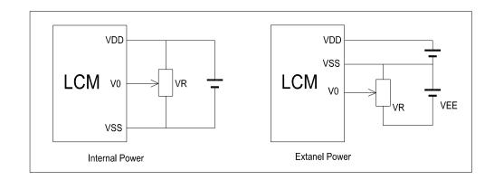
$V_{DD\sim}V_0$ : LCD Driving voltage
