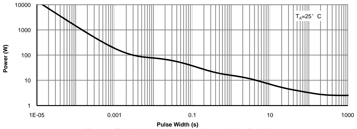
Figure 14: Single Pulse Power Rating Junction-to-Ambient (Note H)
