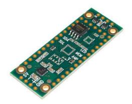
**Description:** This low-cost (LC) Teensy Prop Shield is meant for making light and sound effects on small, handheld props and wearable costumes. This shield features a 2W audio amp, high-speed 5V buffers for driving APA102 LEDs, and an 8MB flash memory. This economical board is approximately the size of a Teensy, just slightly longer to allow space for mounting holes and connections for power, speaker and LEDs.
