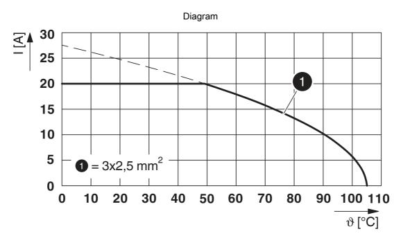
I = current strength,  $\vartheta$  = ambient temperature, 3x 20 A
