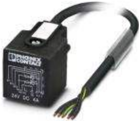
Sensor/Actuator cable, 5-position, PUR halogen-free, Black RAL 9005, Free cable end, on AD valve plug (pressure switch), with 2 LEDs, Cable length: 10 m
