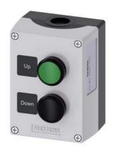
enclosure for command devices, 22 mm, round, enclosure material plastic, enclosure top part gray, 2 control points plastic, B=Pushbutton green, label: Up, 1 NO, screw terminal, A=Pushbutton black, label: Down, 1 NO, screw terminal, floor mounting, 1xM20 each on top and bottom, Labels glued in
